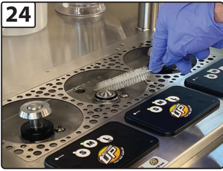
24 SCRUB AROUND EXPOSED VALVES AND RINSE CLEAN
