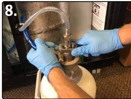
8. TAP CLEANING CANISTER AND WAIT 5 SECONDS FOR PRESSURIZATION
