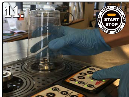
11. HOLD A CUP UPSIDE DOWN OVER THE NOZZLE. THEN PRESS THE START/STOP BUTTON
