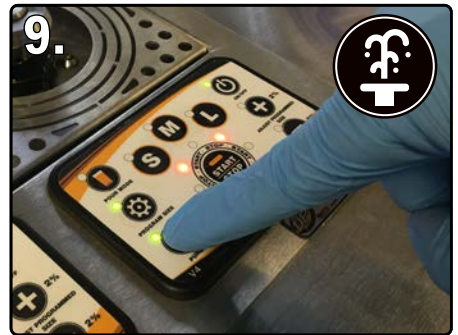
9. PRESS THE PURGE BUTTON ON THE CONTROL PANEL OF THE LINE YOU ARE LOOKING TO CLEAN
