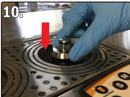
10. AND PUT THE NOZZLE INTO THE DOWN POSITION
