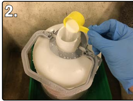
2. POUR BEER LINE CLEANER INTO CANISTER (RATIO IS LOCATED ON LINE CLEANER)
